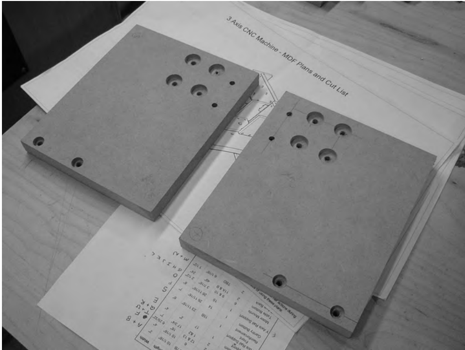
Figure 15-7. Parts W and X drilled with counterbore holes drilled on opposing sides
