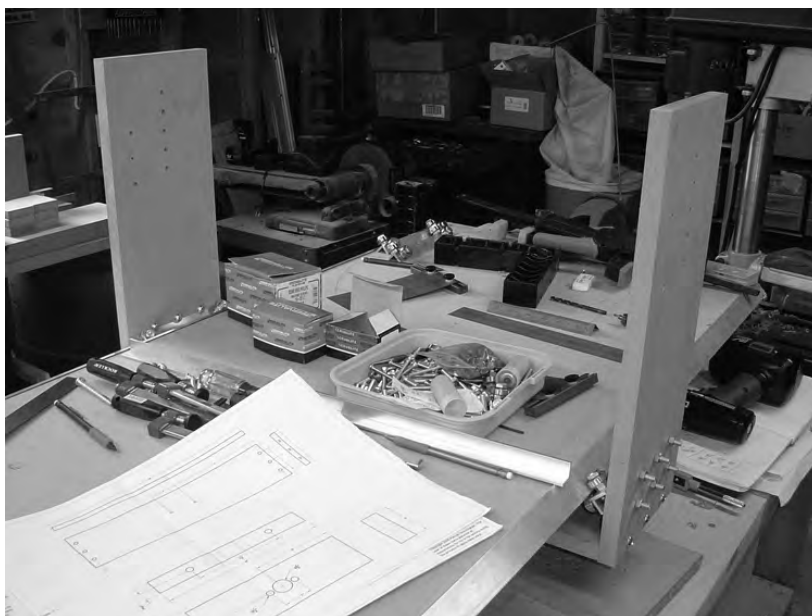
Figure 11-12. Partial frame with gantry sides and bottom installed
