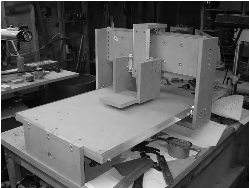
Figure 16-19. Your CNC machine without any electronics
