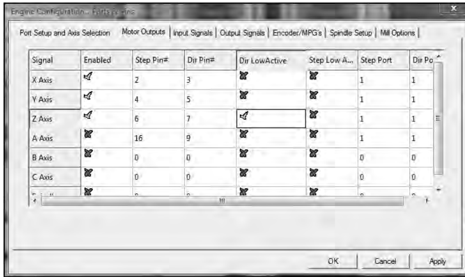
Figure 18-11. Changing a motor's direction of spin is quick and easy.
