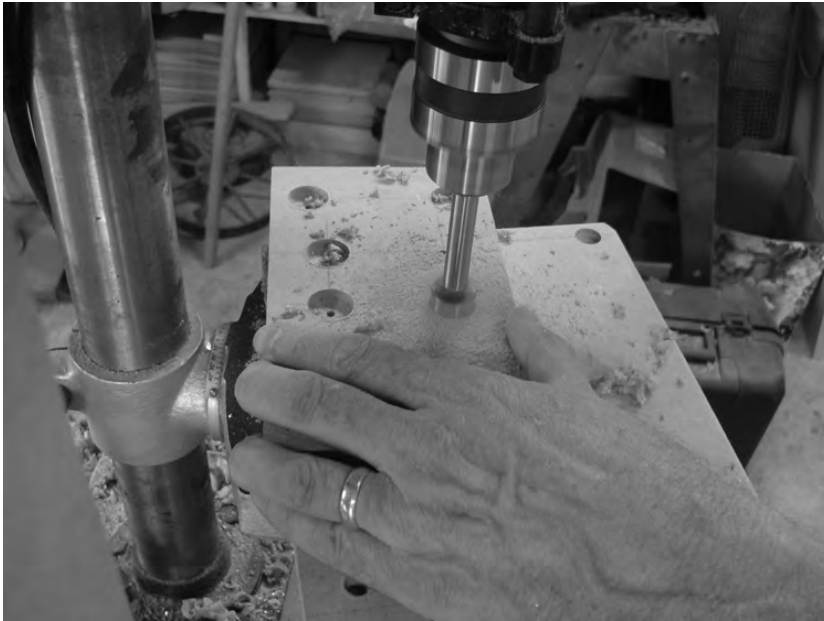
Figure 13-6. Drilling the counterbored holes in Part C
