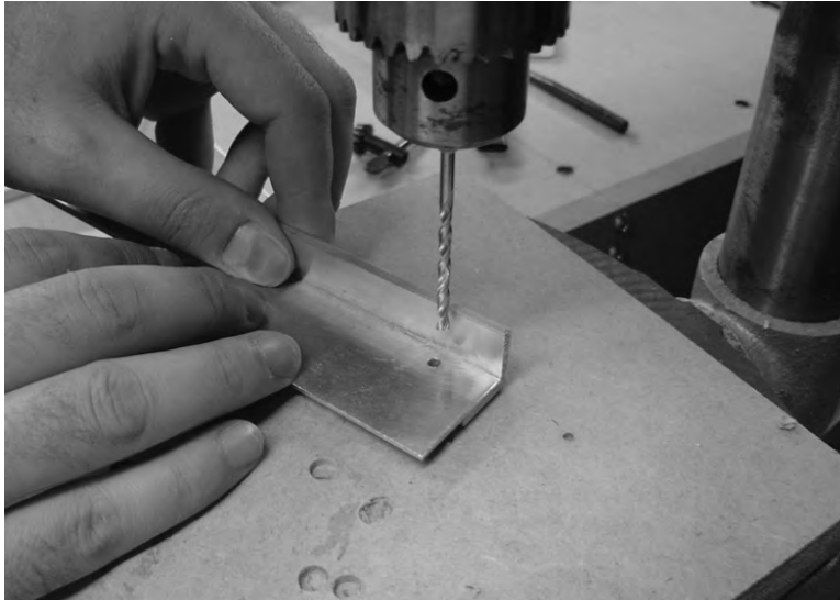
Figure 10-10. Drilling pilot holes into the BRA rails
