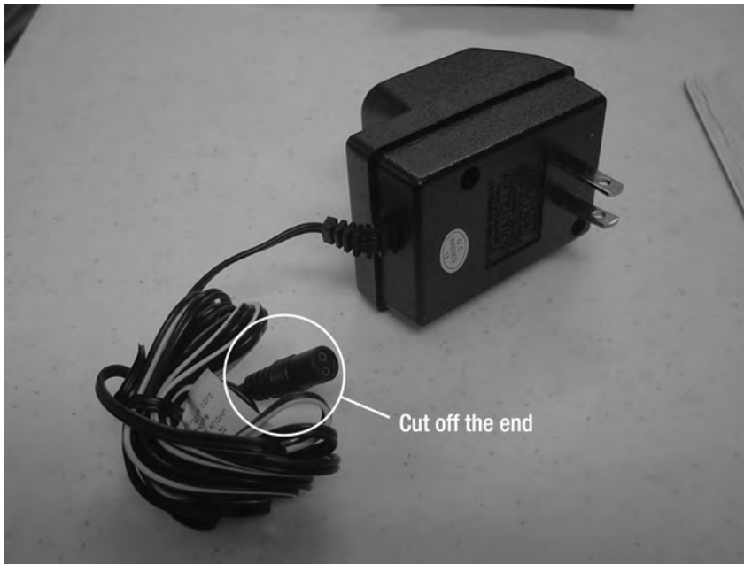
Figure 6-13. A 5- or 6-volt adapter will power the breakout board.
